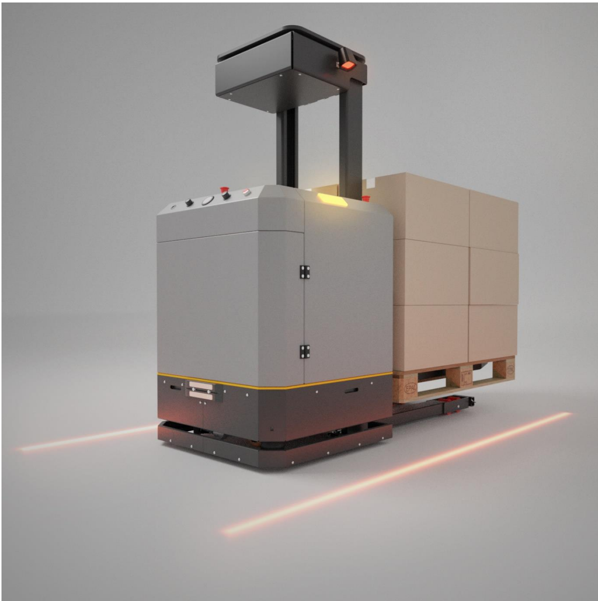
Picture 2: 12 integrated cameras take over the complete navigation of the AGV and provide millimeter precision (source Logivations)
